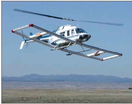
Figure 8. ORAGS-TEM system in transit near the Black Hills, South Dakota.
